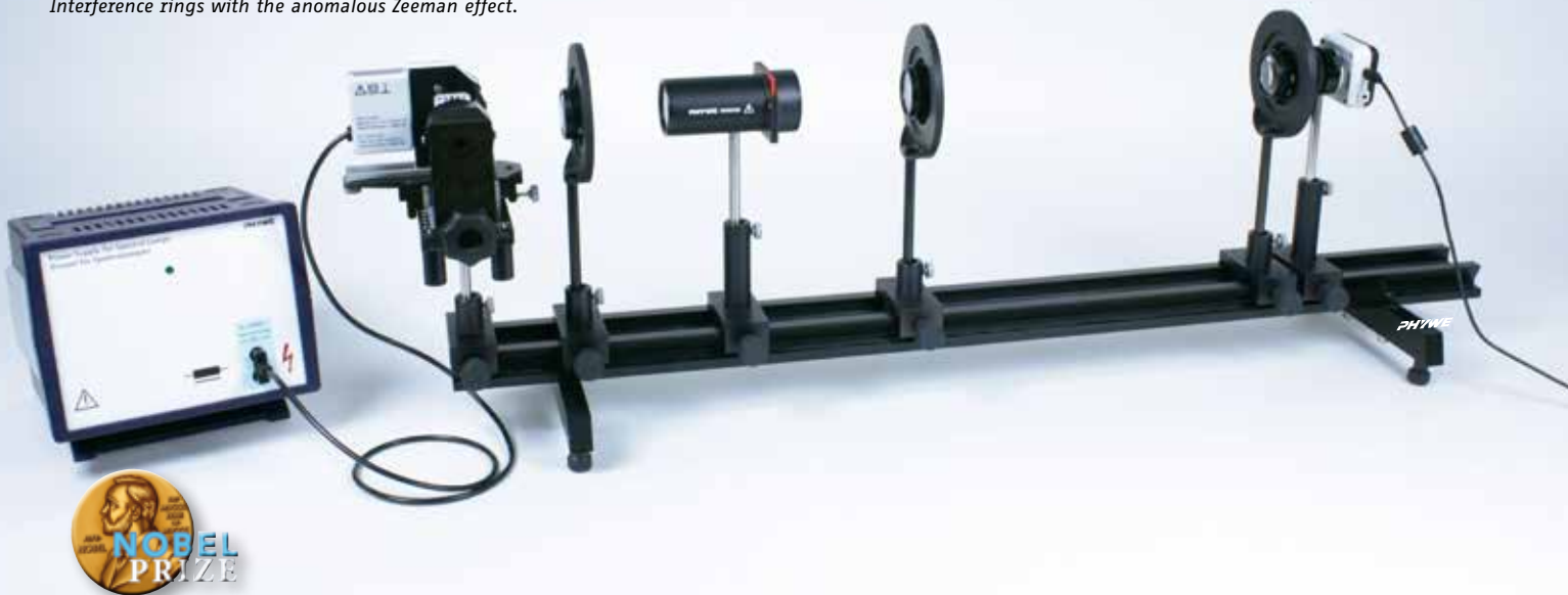
Interference rings with the anomalous Zeeman effect.
