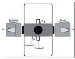
Schematic set-up with an indication of the angular positions.
