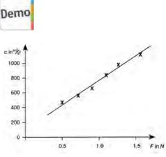
The square of phase velocity depending upon the force  $\mathcal{F}$  applied on the rope.
