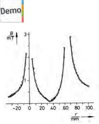
Magnetic field component By of two parallel conductors on the x-axis as a function of the distance from one conductor, if the current in both conductors is in the same direction.
