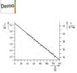
Temperature dependency of surface tension of olive oil.
