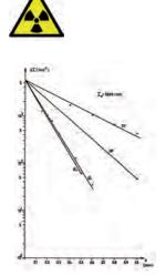
Counting rate I as a function of absorber thickness.
