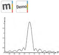
The angular distribution of the intensity of a plane ultrasonic wave diffracted at a slit.
