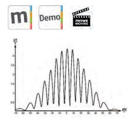
Angular distribution of the intensity of two interfering ultrasonic waves having the same phase, amplitude, frequency and direction of propagation.
