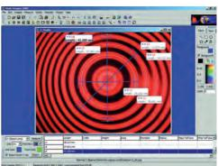
Screenshot of software used to measure the diameters of the interference rings as captured by the CCD-Camera.
