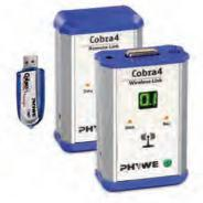
Wireless-Link + Wireless Manager + Remote-Link for wireless measurements
