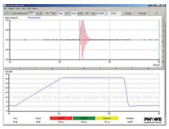
4 MHz probes, cylinder with approx. 120 mm, time-of-flight measurement with zoom on.
