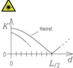
Experimentally determined contrast function in comparison to the theoretical contrast function K of a 2-mode laser.
