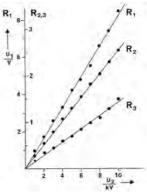
$U_I$  (measured voltage) as a function of  $U_2$  (charging voltage) measured on conducting spheres with three different diameters.
