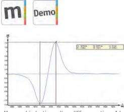
Measured induction voltage USS versus time. Additionally the evaluation of the peak-to-peak voltage USS = 2.766 V is shown.
