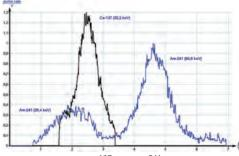
Calibration lines of <sup>137</sup>Cs and <sup>241</sup>Am.
