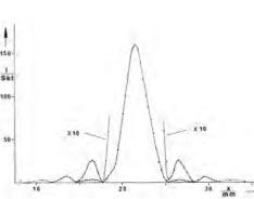
Diffracted intensity I vs position x of the photodiode, using a diaphragm with D1 = 0.25 mm.
