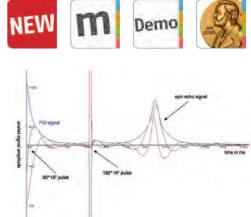
Spin echo signal of an oil sample occuring 10 ms (echo time) after a 90° HF pulse (FID signal is shown). To generate the echo signal a 180° HF pulse has to be switched after half the echo time.
