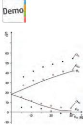
Temperatures at the inlet and outlet of the vaporiser  $V_i$ ,  $V_0$  and condenser  $C_i$ ,  $C_0$  as a function of the operating time; continuous curves: temperature in water reservoirs.
