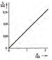
Torque and deflection of a torsion bar.
