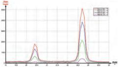
X-ray spectrum at different anode voltages.
