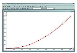
Height of fall as a function of falling time.
