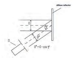
Diagram of the principle of measurements with the used magnitudes (with  $\mathcal{O}^*$  as apparent magnitude of surface  $\partial$ ).
