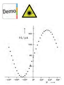
Corrected photo cell current as a function of the angular position of the polarization plane of the analyzer.
