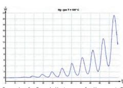
Example of a Franck-Hertz curve for Hg-gas at T = 180 °C.
