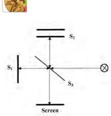
Beam path in Michelson's interferometer.
