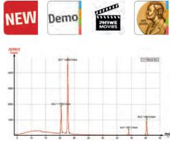
Intensity of the X-radiation of copper as a function of the glancing angle theta; analyser crystal: LiF.
