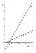
Temperature differences measured at various ram pressures.
