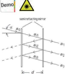
Multibeam interferometer after Fabry and Perot. Illustration of the principle for deriving the individual amplitudes.
