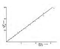
Linear function to determine the horizontal component hBE of the magnetic flux density of the earth-magnetic field.
