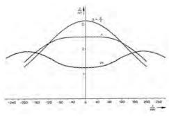
B (r = 0; r is the distance perpendicular to the axis of the coils) as a function of z (z is the distance from the center of the coils in the direction of the axis of the coils) with the parameter.
