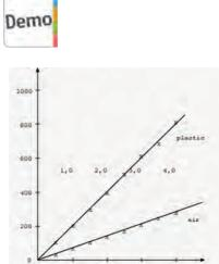
Electrostatic charge Q of a plate capacitor as a function of the applied voltage  $U_c$ , with and without dielectric (plastic) between the plates ( $\alpha$  = 0.98 cm).
