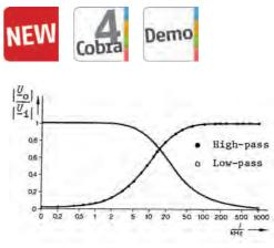
Example of a measured frequency response of the high- and low-pass filters.
