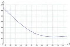
Total gamma-absorption coefficient as a function of the energy.
