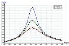
Total voltage as a function of frequency in the parallel tuned circuit. Curves recorded for different resistors (top down):  $R = \infty \Omega$ , 1000  $\Omega$ , 470 Ω.
