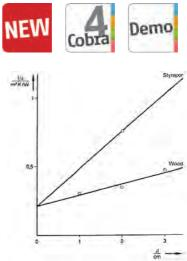
Heat transition resistance 1/k as a function of the wall thickness d.
