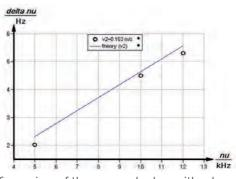
Comparison of the measured values with calculated values for a detector moving towards the emitter.
