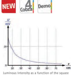
Luminous intensity as a function of the square of the reciprocal of the distance (lamp - diode).
