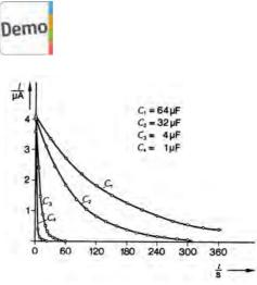
Course of current with time at different capacitance values; voltage and resistance are constant (U = 9 V, R = 2.2 M).
