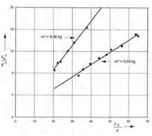
Determination of the momentum of inertia from the slope of straight line  $(tR)^{-1} = f(tP)$ .
