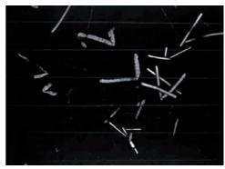
Particles visible in the diffusion cloud chamber.
