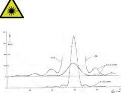
Diffraction intensity I as a function of location x for the single slit b1 = 0.1 mm and b2 = 0.2 mm. The x axis of the graph for b1 = 0.1 mm is shifted upwards. The intensity of the areas next to the central peak is represented enlarged by a factor of 10. (Distance between slit and photodiode L = 107 cm; = 632.8 nm).
