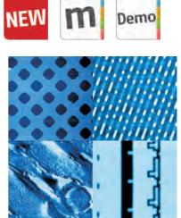
Topography of microstructure (50  $\mu$ m), CD stamper (20  $\mu$ m), skin cross-section (60  $\mu$ m), and SCA chip structure (40  $\mu$ m) FLTR.
