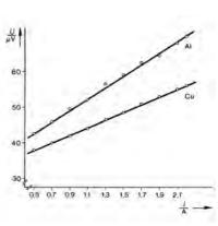
Current/voltage characteristics of a copper rod and an aluminium rod.
