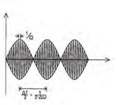
Resulting difference signal during interferometric measurement.
