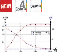
Voltage ratio (left axis) and phase displacement (right axis) of the double CR network as a function of frequency with  $R_1$ =50  $\Omega$ ,  $R_2$ =1 k $\Omega$  and  $C_1$ =25 µF,  $C_2$ =50 µF.
