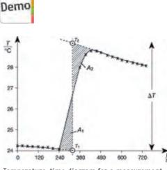
Temperature-time diagram for a measurement example.
