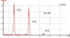
Bragg reflexes with an increasing order of diffraction at theta = 24°.
