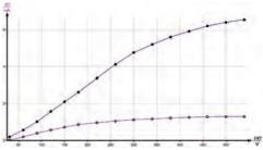
Ionisation current I<sub>C</sub> as a function of the capacitor voltage  $U_C$  for different diaphragm tubes.
