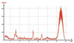
Characteristic fluorescence spectrum of the detector components (energy of the primary radiation  $E_0 = 32.5$  keV).
