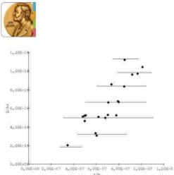
Measurements on various droplets for determining the elementary charge by the Millikan method.
