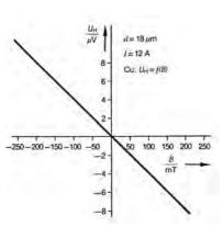
Hall voltage as a function of magnetic induction B, using a copper sample.
