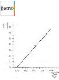
Example of a measurement: boiling point increase as function of concentration of table salt in an aqueous solution.
