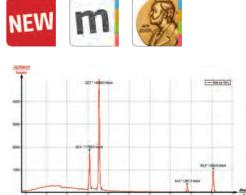
Intensity of the X-radiation of copper as a function of the glancing angle theta; analyser crystal: LiF.
