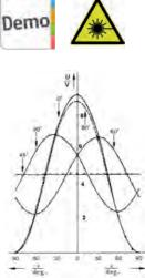
Intensity distribution of polarised light for different angles of the /4 plate, as a function of the analyser position.
