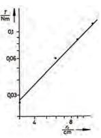
Moment as a function of the distance between the origin of the coordinates and the point of action of the force.
