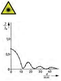
Intensity distribution for diffraction through a slit as a function of the location along a straight line running parallel to the plane of the slit, normalised according to intensity  $I_0$  without slit.
