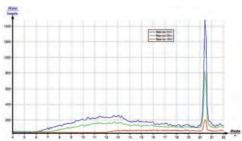
Bremsspectrum of copper for three different anode voltages U (15 kV, 15 kV, and 31 kV), x-axis: glancing angle theta /°.
