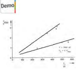
Ripple of the output voltage as a function of the charging current: a) half-wave rectifier, b) bridge rectifier.
