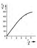
Pump cooling capacity as a function of the operating current.
