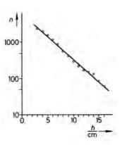
Number of steel balls (m = 0.034 g), as a function of the height h, which pass through the volume element V in 30 seconds (vibrational frequency 50 Hz).
