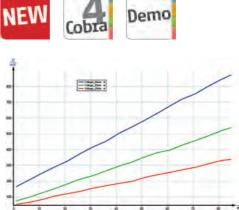
Induced voltage as a function of current for different coils.
