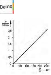
Electric field strength as a function of the plate voltage.
