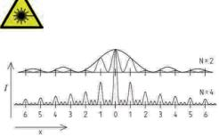
Qualitative intensity distribution of diffraction through 2 and 4 slits, the distance x being normalised to *Is*. The intensity distribution of the simple slit has been represented with exaggerated height to give a clearer view.
