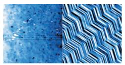
Digital Data Storage (DAT) tape: Topography (left, 50  $\mu$ m) and phase contrast image (right, 50  $\mu$ m) at same location. The phase contrast image contains the magnetic information and shows a stripe-like structure with a mean feature size of 3  $\mu$ m (one bit).
