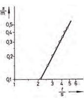
Distance travelled by the centre of gravity of the Maxwell disk as a function of time.
