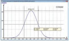
Normal distribution of the iron  $K\alpha$ -lines for determining the line energy and the full width at half maximum (the original measurement curve is hidden).
