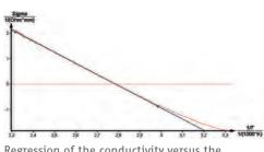
Regression of the conductivity versus the reciprocal of the absolute temperature.
