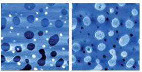
PS/PMMA films: Topography and phase contrast, 3 µm.
