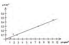
Attenuation coefficient of different materials as a function of the material density (from left to right: Plexiglas®, concrete, aluminium, iron, lead).
