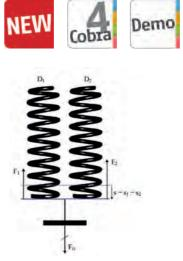
Parallel connection of helical springs.
