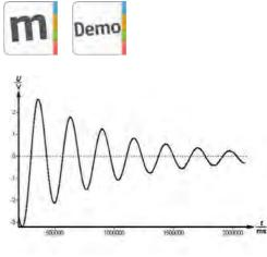
Output voltage of the free and damped oscillating Cavendish balance.
