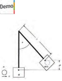
Diagram on the theory of the ballistic pendulum.
