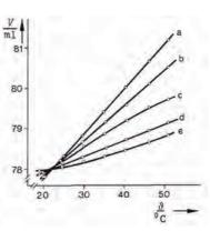
Relationship between volume V and temperature T of: a) ethyl acetate, b) methylated spirit, c) olive oil, d) glycerol and e) water.
