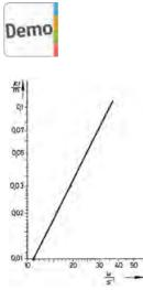
Location of the lowest point c of the liquid as a function of the angular velocity.
