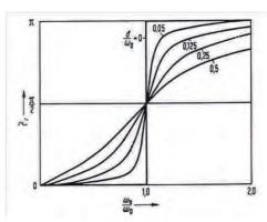
Phase shifting of forced oscillation for different dampings.
