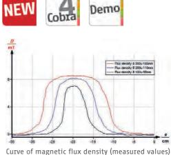
Curve of magnetic flux density (measured values) for coils with a constant density of turns n/l, coils radius r = 20 mm, lengths
