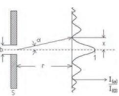
Principle of set up for diffraction through a slit and qualitative distribution on intensities in the detector plane LD.
