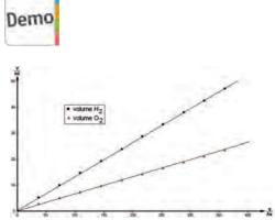
Correlations between the transferred charge and the evolved volumes of hydrogen and oxygen in the electrolysis of diluted sulphuric acid (T = 296.05 K and p = 100.4 kPa).
