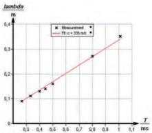
Determination of the velocity of sound at a tube length of /= 615 mm.
