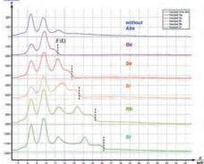
X-ray spectra with the K-absorption edges.
