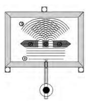
Interference with the double slit.
