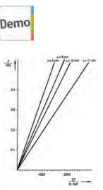
Relationship between electrostatic force F and the square of the charge Q for various distances (a) between ball and plate.
