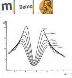
Ionization current as a function of position (u) of detector with large excitation currents in the magnetic analyser.
