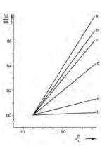
Relationship between length and temperature for a) aluminium, b) brass, c) copper, d) steel, e) duran glass, f) quartz glass (lo = 600 mm).
