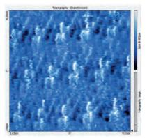
Charge density waves on T<sub>a</sub>S<sub>2</sub>.
