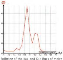
Splitting of the Ka1 and Ka2 lines of molybdenum (n = 4)
