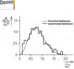
Experimental and theoretical velocity distribution in the model experiment.
