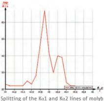
Splitting of the Ka1 and Ka2 lines of molybdenum (n = 4)
