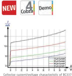
Collector current/voltage characteristic of BC337 transistor.
