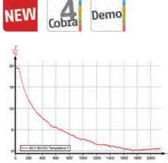
Temperature curve of the water during pumping. The boiling temperature of water is dependent on the pressure of the air that burdens it.
