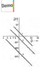
Precession frequency as a function of the gyro frequency for different additional masses.
