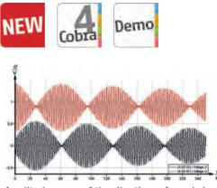
Amplitude curves of the vibrations of coupled pendula in the beat case for three different coupling lengths I = 30 cm.
