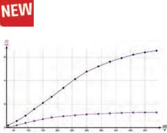
Ionisation current Ic as a function of the capacitor voltage Uc for diffrent diaphragm tubes.
