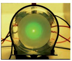
Interference rings of graphite on a fluorescent screen.
